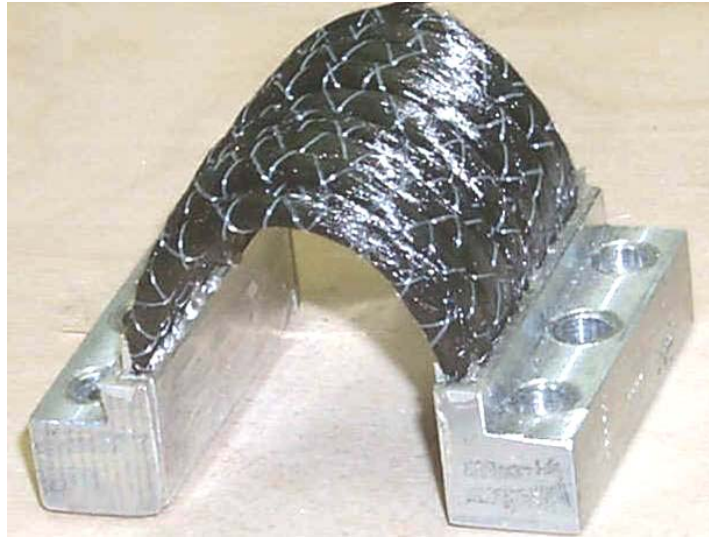
Figure 3. U-shaped GFTS for minimal force and vibration transmission.
