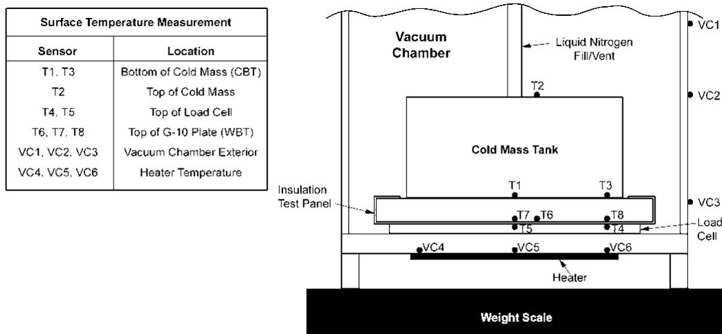
**FIGURE 6.** Simplified schematic of Cryostat-5 test assembly showing temperature sensor locations
