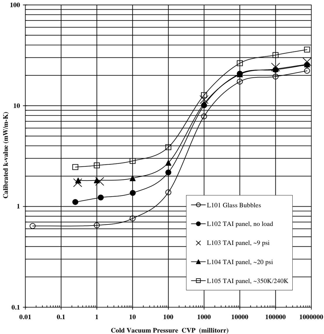
FIGURE 7. Calibrated k-value variation with vacuum pressure. Boundary temperatures are 293 K and 78 K
