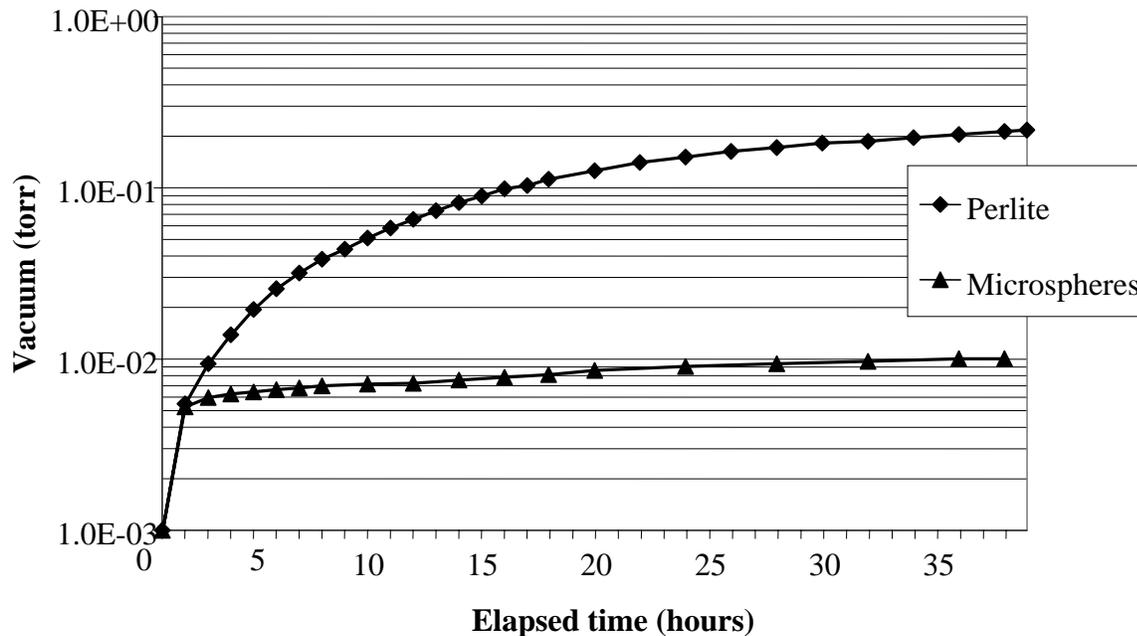
**FIGURE 2.** Vacuum decay comparison
