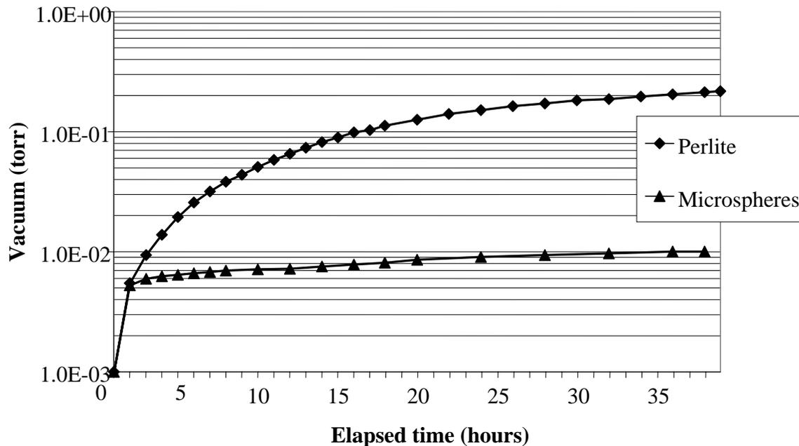
**FIGURE 2.** Vacuum decay comparison
