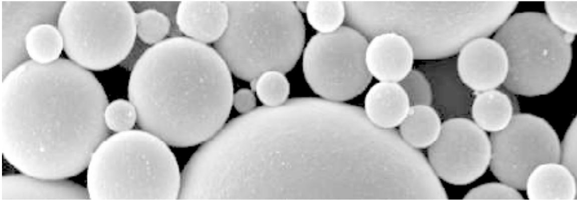
**FIGURE 1.** Microspheres magnified 500x
