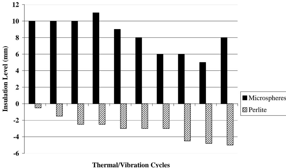
FIGURE 3. Microsphere and perlite insulation level change following thermal/vibration cycles
